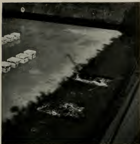
View of flow to pump intakes at low dock water level.
